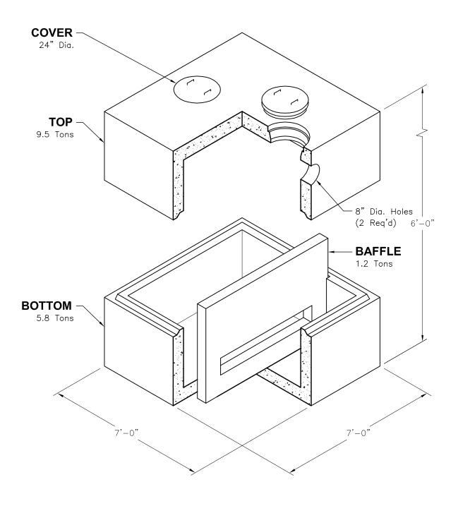
This print is an example of an o/w separator and is not designed for specific performance ratings. Openings can be modified for specific project requirements.
