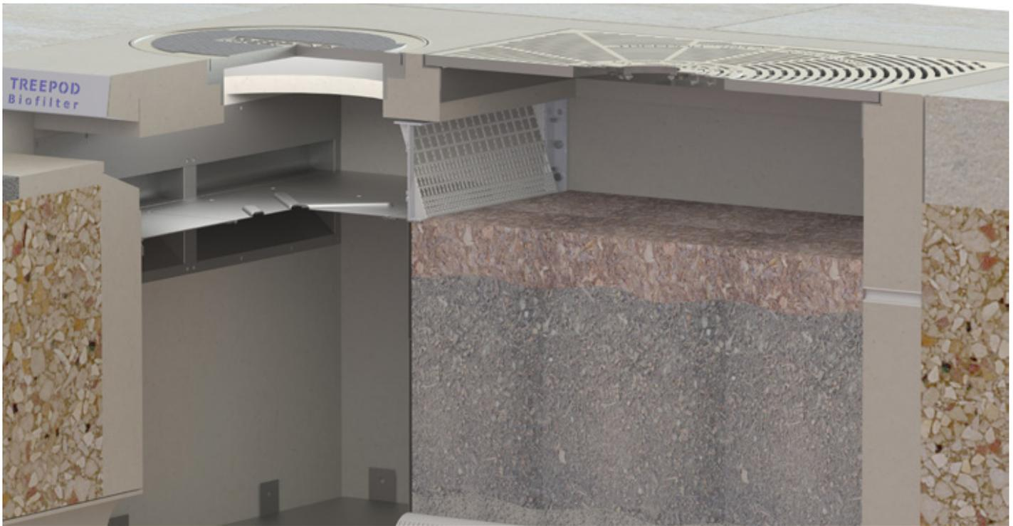
Cutaway illustration of a BioPod biofiltration unit. Pollutant-heavy stormwater runoff enters the curb inlet at the top. Large debris collects in the pretreatment chamber. As water travels downward, pollutants are filtered out by planting media. The tree gets water and nutrients from the collected runoff. Filtered water is collected by the perforated pipe at the bottom and carried out of the unit to the drainage system.
