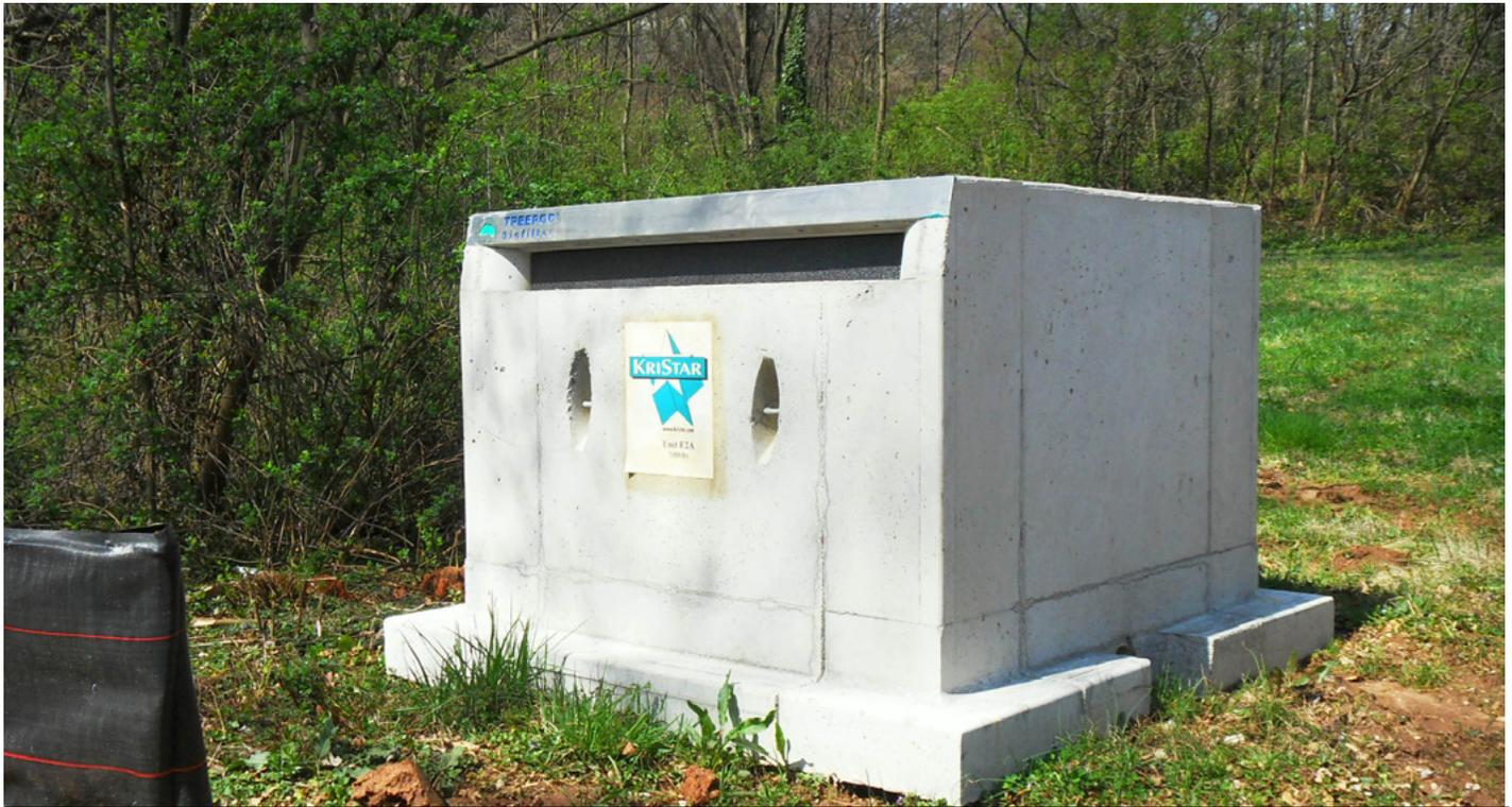
A 4' x 4' BioPod unit, as delivered to the jobsite. The concrete biofiltration unit will be buried so the top is flush with the sidewalk, aligning the bottom of the curb inlet with the road bed.
